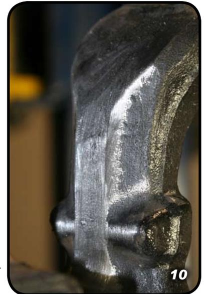
19. Tack the gusset on in a few places on either side so it does not move when you start your welding process.
