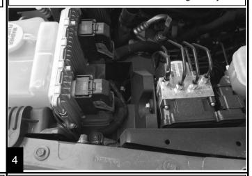
With a 10mm loosen the ABS module bolt enough to slide the forked end of the ARB bracket between the head of the bolt and the bushing. Also, remove the left side fender bolt that is located 4th from the back of the engine bay.
