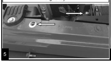
Slide the forked end of the bracket over the ABS module bolt and loosely install the fender bolt through the tab of the ARB bracket.
