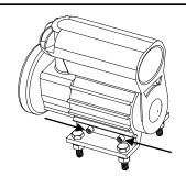
Using the hardware supplied with the ARB compressor, mount the compressor to the Base Plate. Note Orientation. Tighten using a 10mm.
