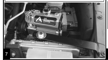
Make sure the compressor and the bracket clear all surrounding components and tighten the 7/16" hardware using a 5/8" and tighten the fender bolt with a 10mm.
