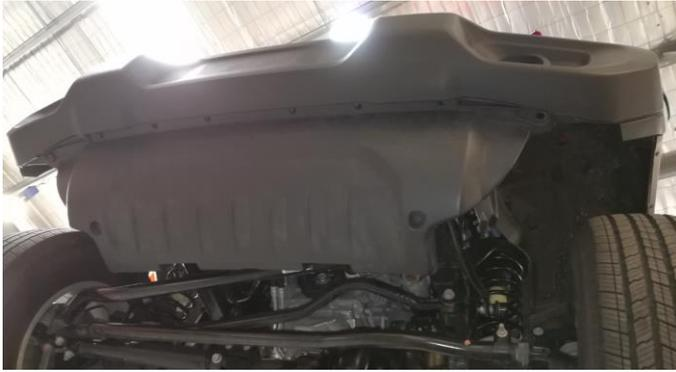
1. Remove plastic splash panel from underneath bumper by removing 2 lower screws and prying apart 8 plastic grommets,
