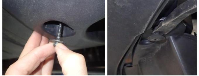
For Rubicon vehicles fitted with steel under panel, remove by unbolting from chassis brackets and lower edge of steel bumper.
