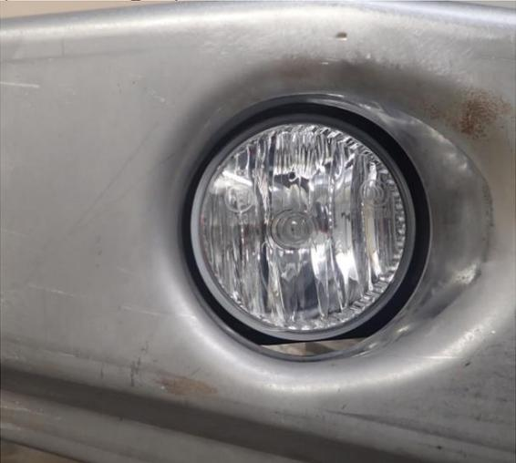
15. Adjust fog light so that it sits central to the fog light aperture in the bull bar. Tighten both bolts on each side of bar to torque specification.
