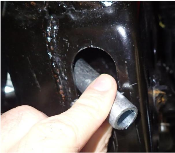
21. Assemble M12x82mm crush tube into lower section of chassis rail via the opening at the front.
