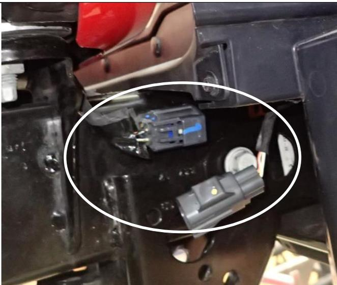
3. Disconnect fog light harness, located on the RHS chassis rail, access from wheel arch.
