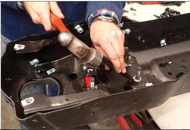
5. For Rubicon vehicles fitted with steel bumper, impact beam is a two piece design; use a chisel to remove lock washers to disassemble from bumper.
