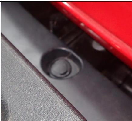
4. Remove 2 plastic grommets from top of bumper with flat bladed screw driver.
