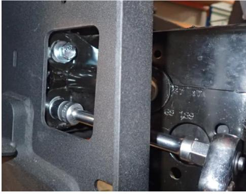
20. Loosely fasten bull bar to vehicle chassis using M10 sems fasteners supplied in chassis mounting kit.
