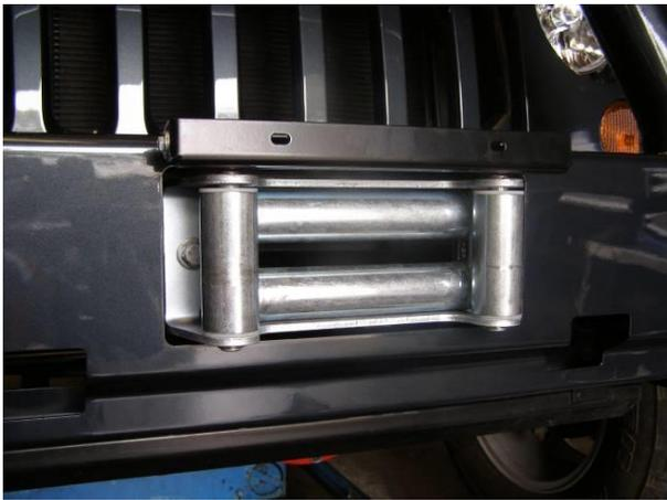
30. Fit the roller fair lead/hawse to the bull bar using M10 or 3/8" fasteners supplied with winch fitment kit.
