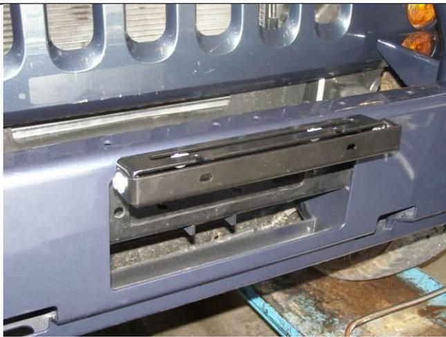
25. Mount number plate bracket assembly to bull bar using M6 fasteners supplied with number plate fitting kit.
