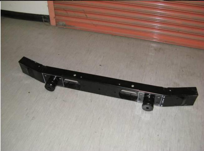
7. Remove steel impact beam from bumper.
