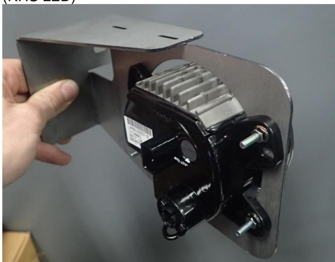
13. Secure front of fog light to rear of mounting bracket using M4 fasteners supplied with fitting kit.
