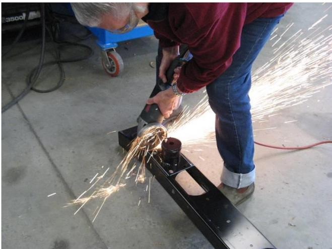
9. Carefully cut marked section using an angle grinder fitted with a cutting disc.
