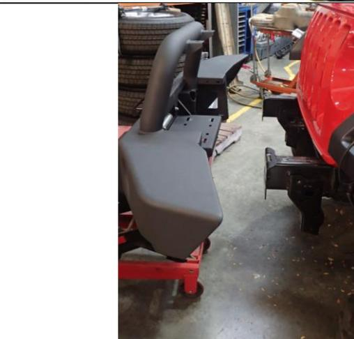
19. With the assistance of a friend or lifting device, present the deluxe bar to the vehicle.
