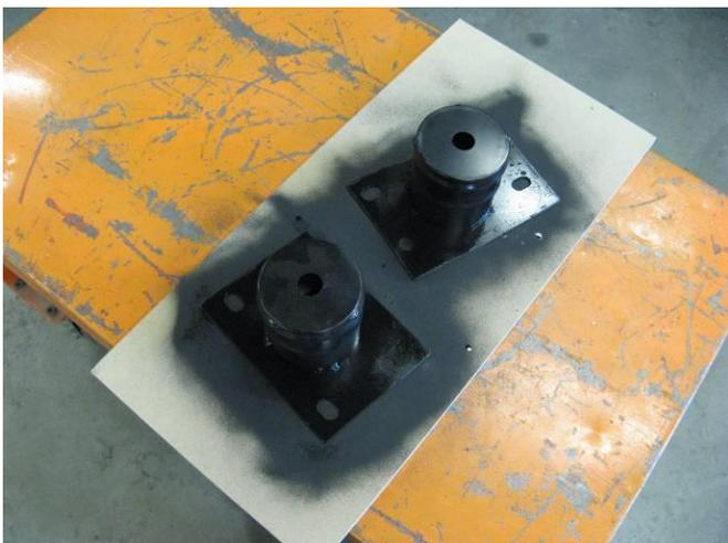
10. Retain crush cans and dispose of the Impact beam.
