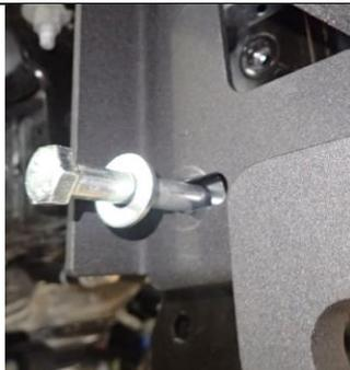
22. Position spacer in between bull bar mounting bracket and chassis
