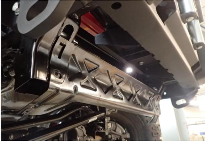
31. Refit OEM front stone panel with original fasteners which were removed in step 2.
