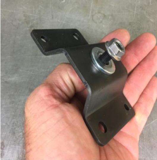
Insert the M8 knurled stud into the awning bracket in the direction shown.
