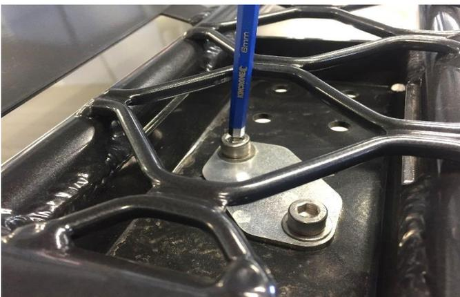
Remove the 2 capscrews securing the roof rack to the mounting bracket.
