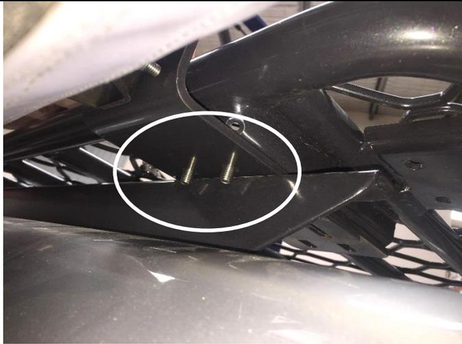
In some installations, the awning bracket may overhang the roof rack support bracket. For these installations install 2 x M8 x 20 capscrews and M8 nyloc nuts with flat washers under each to the 2 outermost holes in the awning bracket and roof rack to add extra support.
