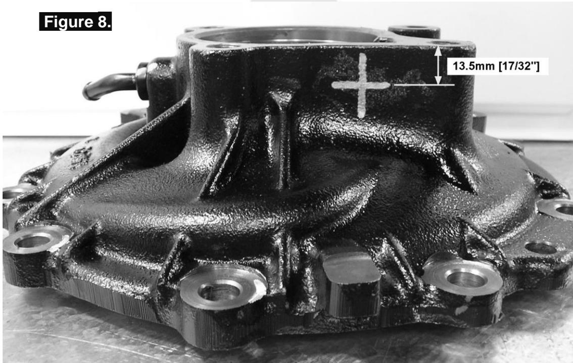
**NOTE :** To best determine the correct vertical position of the drilled hole, measure down from the machined face (shown at the top of the picture in Figure 8.) a distance of 13.5mm [17/32"] and mark the horizontal line which the hole is centered on. Then refer to Figure 9. for the correct position on that line to start drilling.
