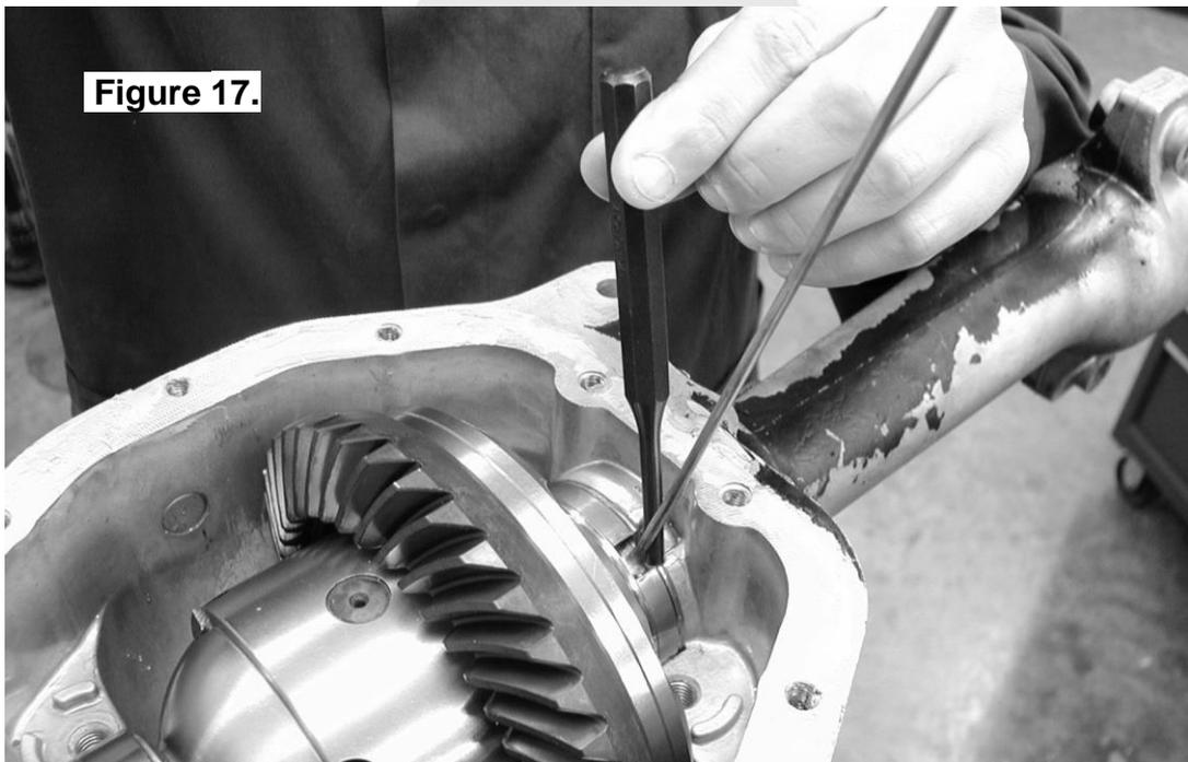
**NOTE :** Do not spread the housing on the aluminum models.
