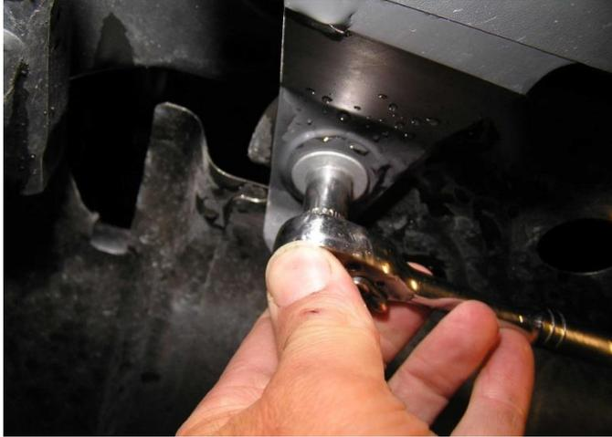
2. Remove lower bumper retaining screws.
