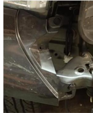
30. Fit pinch weld to both sides along cut edge.
