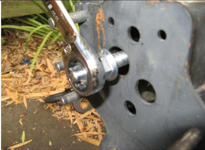
19. Install the chassis stud by fitting 2 nuts to the end of the stud and tightening until thread bottoms out.
