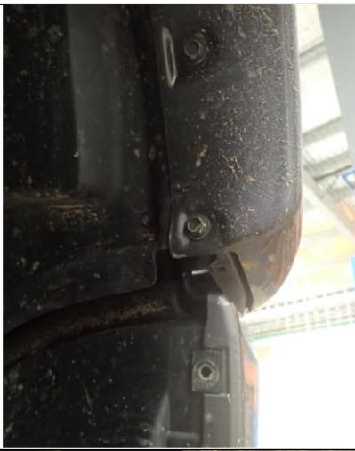
4. Remove upper fender liner retaining screws.
