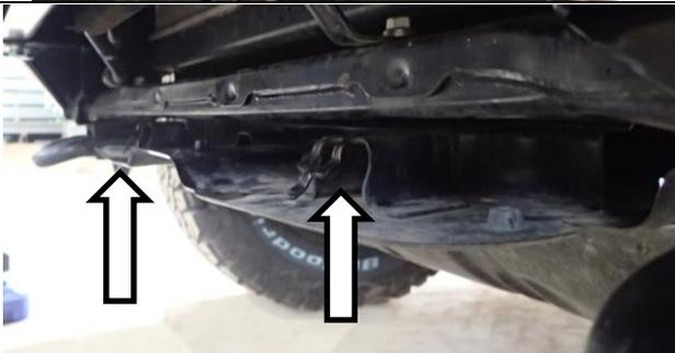
77. In order to allow fitment of the centre stone panel, loosen the front two fasteners of the OEM sump guard several turns.
