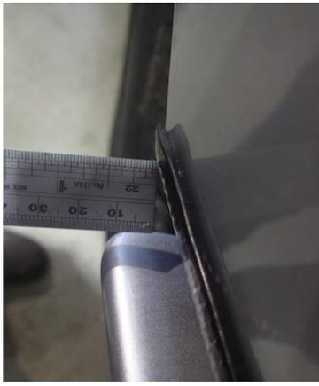
67. Measure the clearance between the RH vehicle fender and the RH bull-bar wing. Repeat on the LH side to confirm the bar is sitting centrally on the vehicle.
