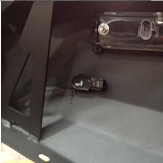
61. Using a small amount of adhesive silicone on the inside surface of the sensor (to prevent rotation). Clip the parking sensor into place from the front of the bullbar. Ensure the sensor connector is facing the correct direction as indicated in the picture.
