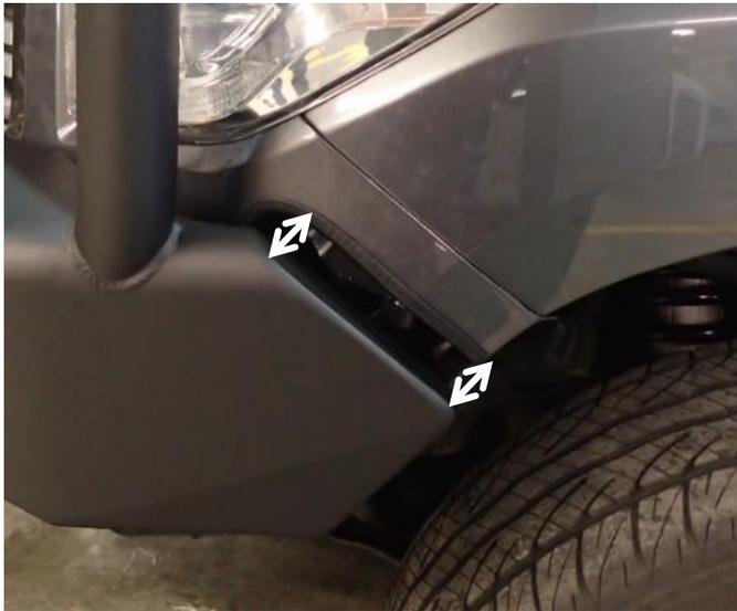
65. Align rear edge of wings with bumper cut profile, so that there is a parallel 18-20mm gap
