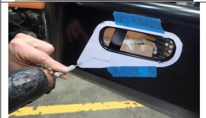
55. Using a centre punch and hammer, mark the drilling hole as shown.
