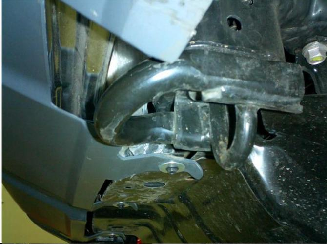
1. Remove tow hooks and bolts, set aside to be refitted.
