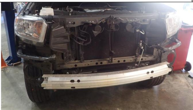
11. Remove all remaining fasteners from lower bumper section.
