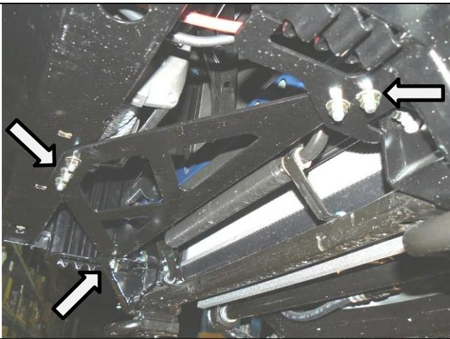
73. Fit the cross brace to underside of lower pan and on top of gussets of mount brackets. Use M10 x 30mm bolts, washers and flange nuts.
