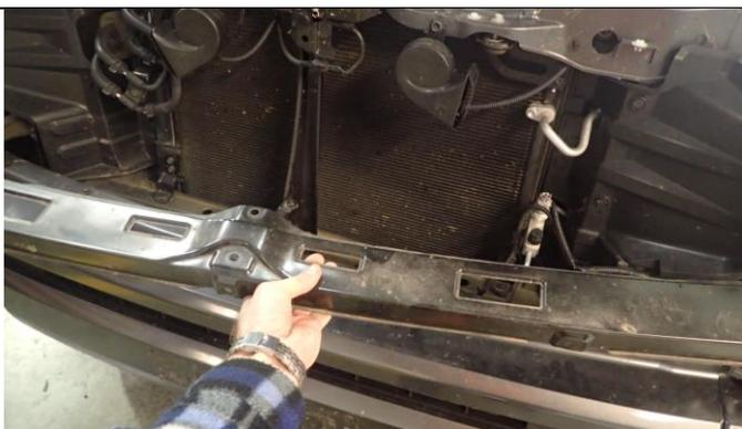
7. Temporarily unbolt grille retaining bracket to access scrivets. This is done by unscrewing nuts from studs.
