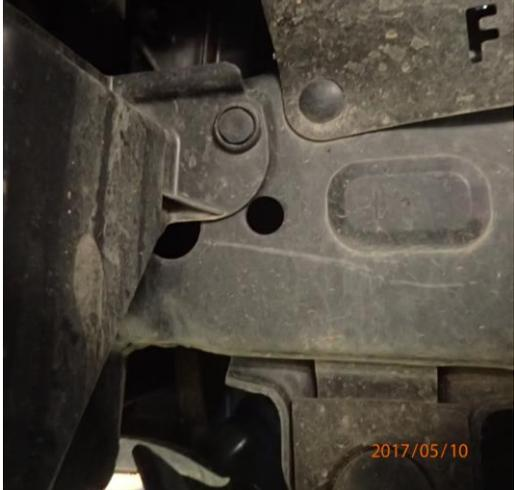
5. Prise out lower fender liner plastic scrivet. Remove lower fender liner completely, they will not be reused.
