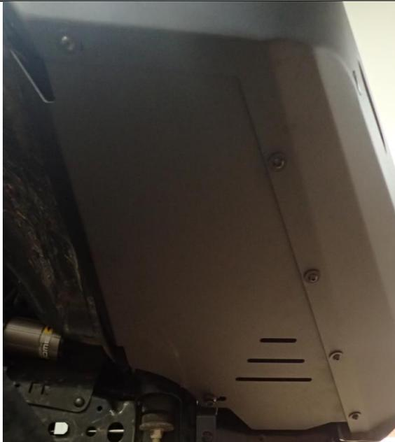
75. Fit 5 x M6 cage nuts to each wing splash panel as shown on **inside** faces.
