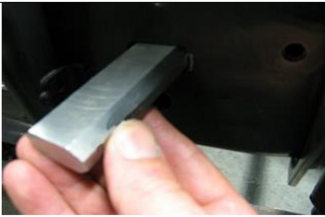
18. Insert clevis nut into rectangular hole in the inboard face of chassis, ensuring the threaded end is inserted first.
