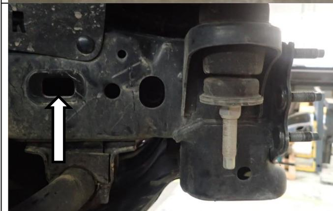
16. Remove rectangular chassis grommets (4) to reveal rectangular cut out in chassis.
