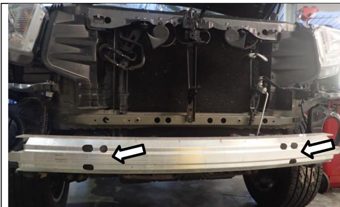
14. Undo fasteners holding Aluminium crash beam to chassis and remove.
