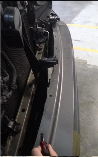
8. Remove all fasteners from top of lower bumper.
