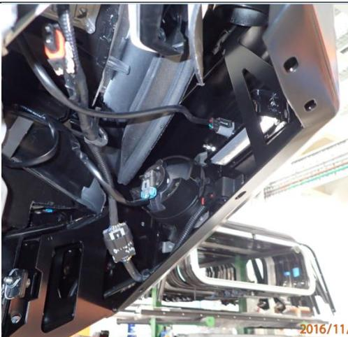
72. Connect electrical plugs for parking sensors, fog lights, driving lights and indicators.
