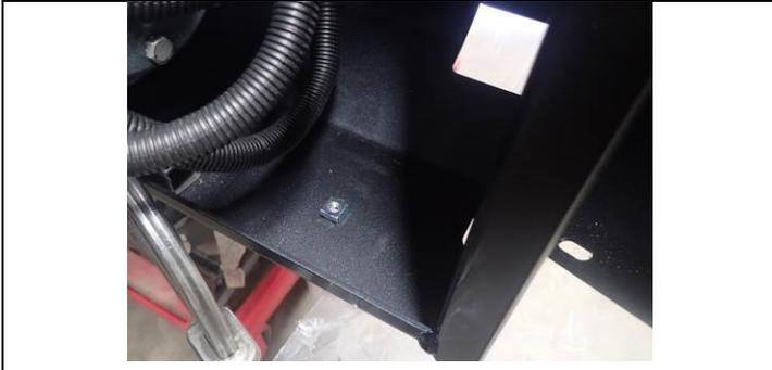
50. Fit the 4 longer leg M6 cage nuts to the lower pan of the bull bar as shown.
