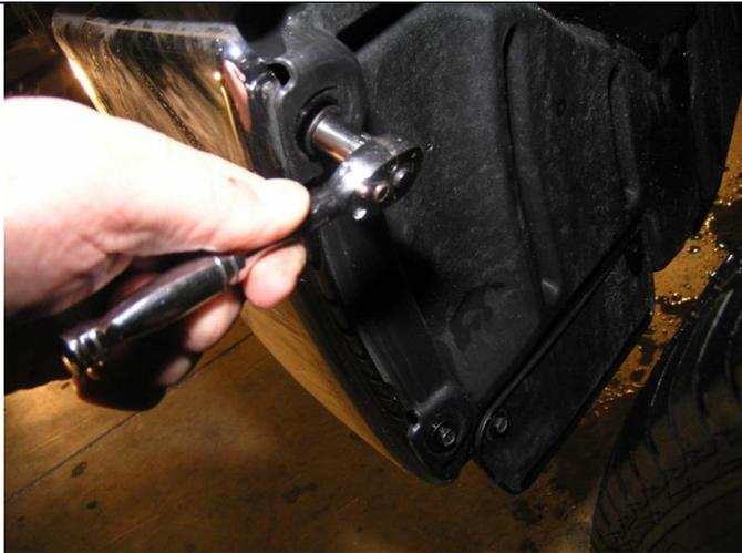
3. Remove all lower fender liner retaining screws to bumper.
