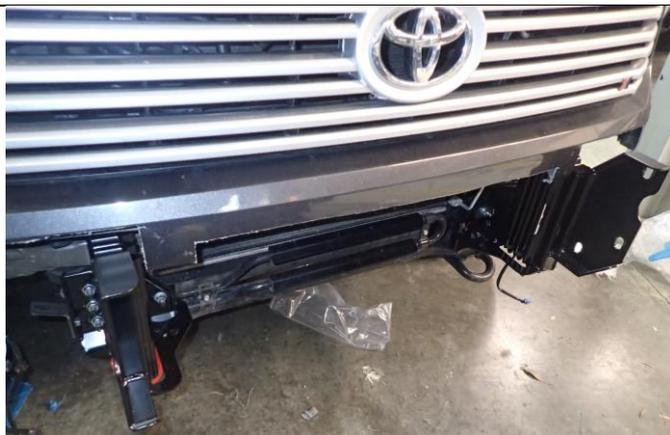
33. Refit grille to vehicle using scriveners and fasteners removed in previous steps.
