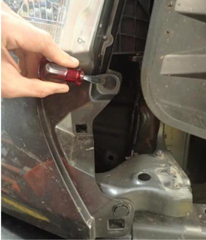
9. Remove screws from trim pieces underneath head lamps.
