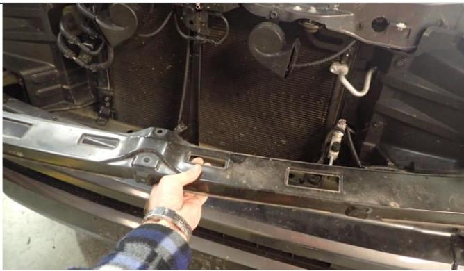
24. Refit grille retaining bracket removed in step 7.
